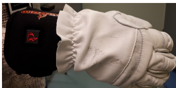
Figure 31. Commercial heating glove covered with the leather outer glove without liner.
