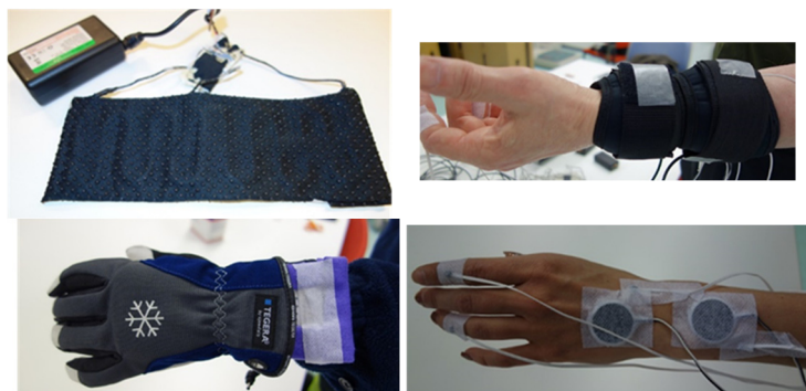
Figure 21. FIR heating pads for hand and wrist (upper panel), protective glove above the pads (lower left) and location of thermistors and heat flux transducers (lower right).
