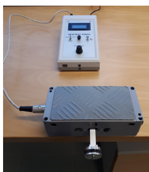
Figure 18. Key grip force test.
