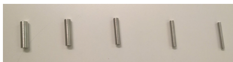
Figure 20. Dexterity test according to EN 420.
