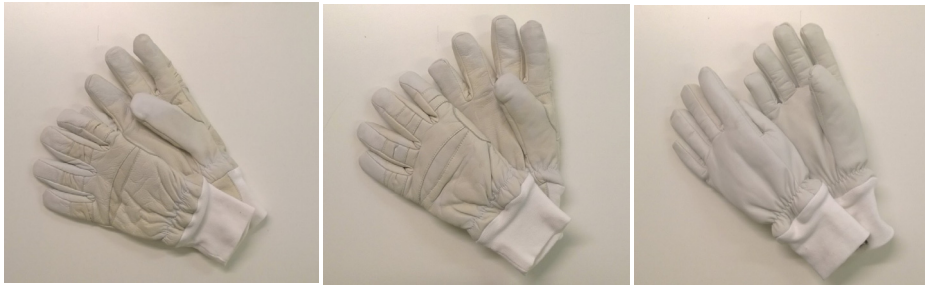
Figure 8. Develop prototypes of the unheated gloves: H1) Already existing product by B. Huhta (Falcon), H2) Added insulation padding on back side of the glove, and H3) Added insulation padding on glove's both sides equally
