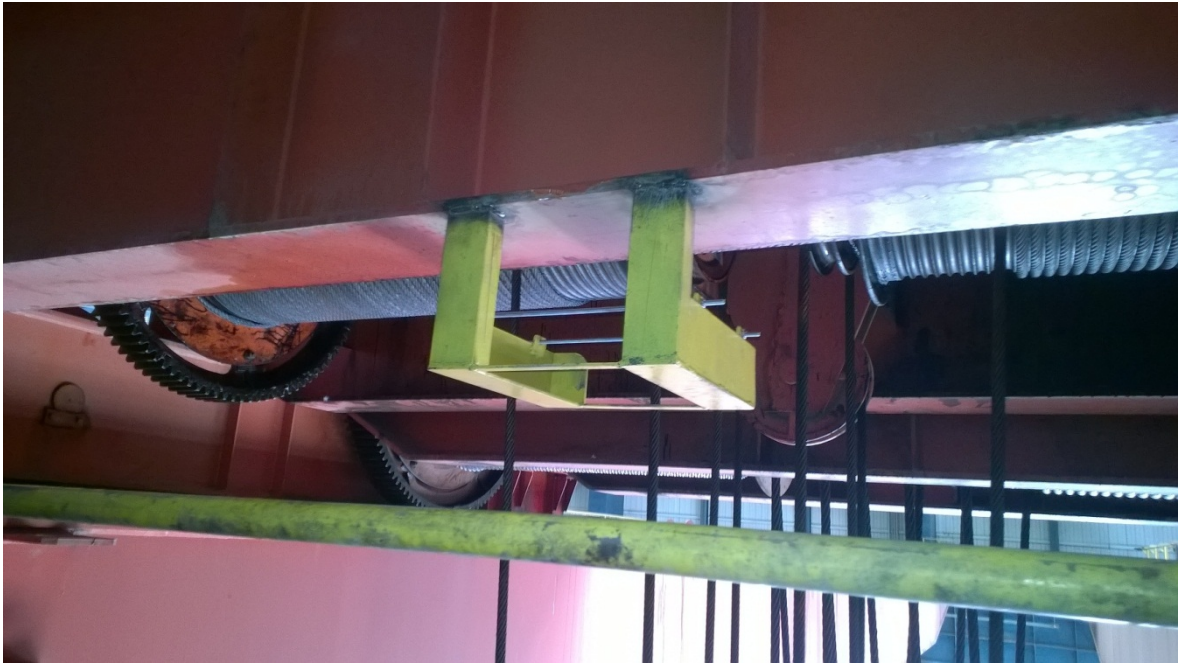
Figure 21. Metallic support for the prototype positioning.
