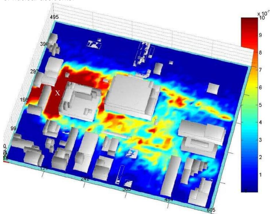
Figure 10 Example of Lagrangian dispersion approach as used in Quic-Plume
