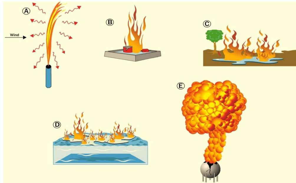
Figure 2 Typical fire phenomena: jet fire, pool fire (in tank pit, freely spreading, on water) and a BLEVE fireball
