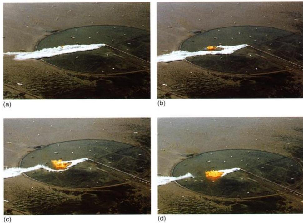
Figure 4 Flash fire upon ignition of a flammable cloud, the flame potentially travels back to the source creating a jet fire (Maplin sands trails, reproduced by permission of Shell research)
