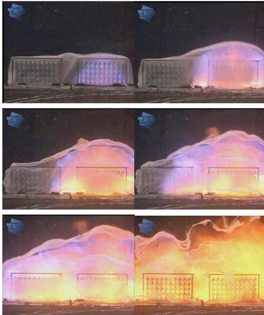
Figure 12 Vapour cloud explosion test performed at TNO with typical congestion structures
