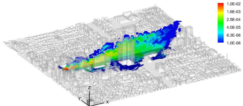
Figure 11 Example of Eulerian CFD dispersion calculation
