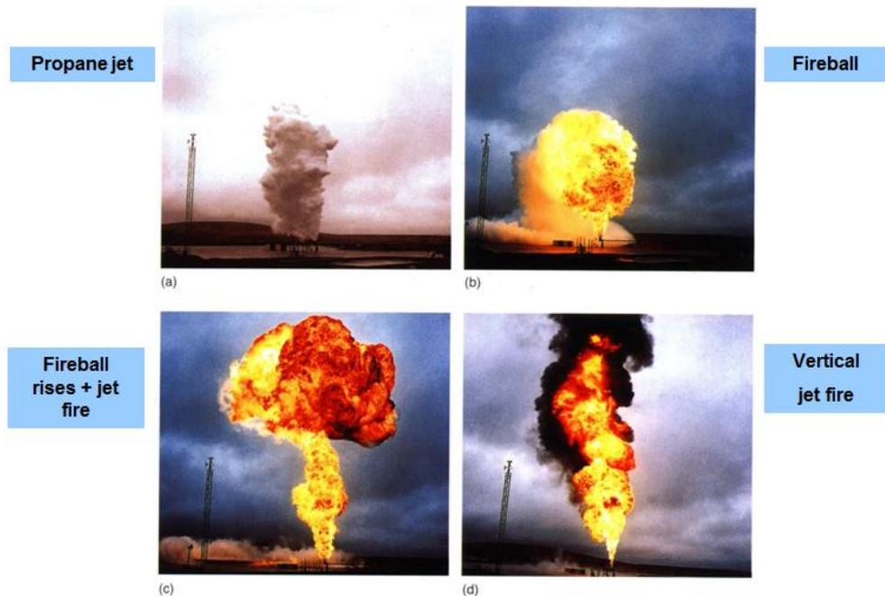
Figure 3 Leak, ignition and resulting fireball and jet fire for a propane release
