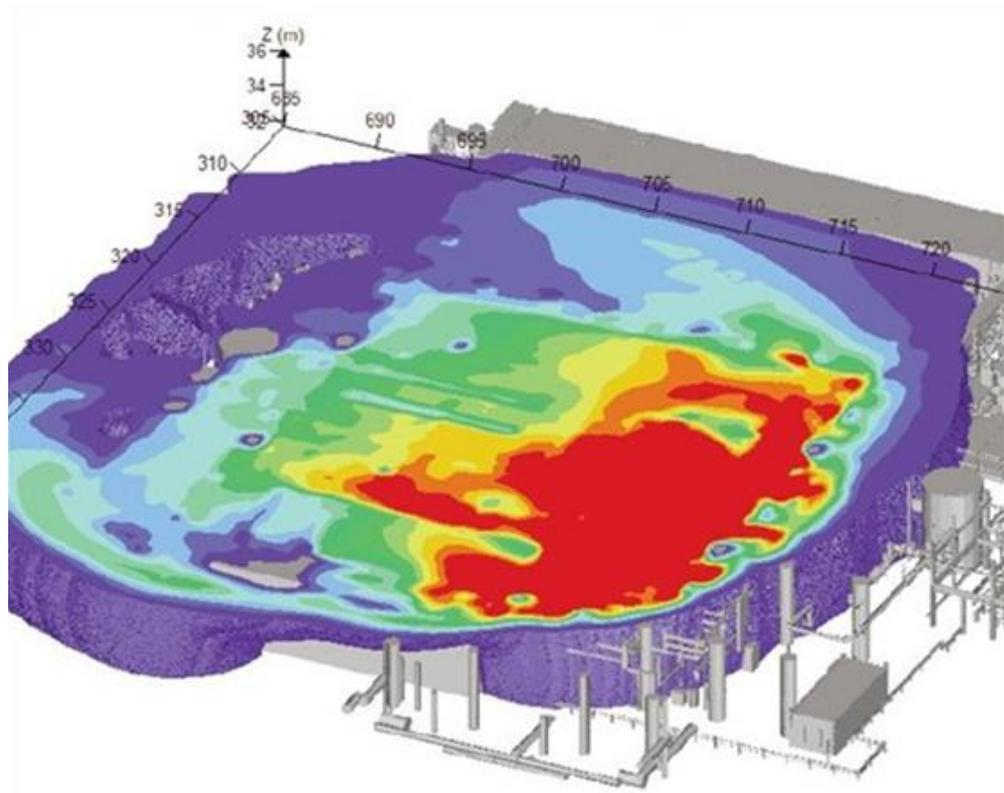
Figure 6 Typical result of a CFD based flammable cloud and VCE overpressure calculation
