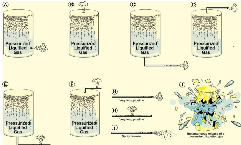
Figure 1 Illustration of various modes of release for a pressurised liquefied gas
